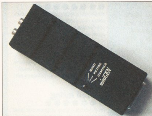
Lola's MiniGen is a basic genlock with a toggle switch – easy to use, good quality, just no RGB pass-through.
